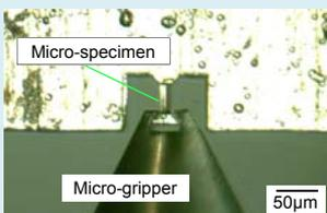
Optical image of the micro-gripper and micro-specimen during the micro-tensile test
