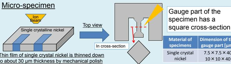
Thin film of single crystal nickel is thinned down to about 30 μm thickness by mechanical polish
