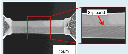
Similar to work reported on tensile testing of single crystal copper micro-specimen [D. Kiener, W. Grosinger, G. Dehm and R. Pippan, Acta Materialia 56 (2008) 580-592]
