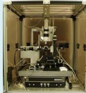
Test machine designed for micro-sized specimens
