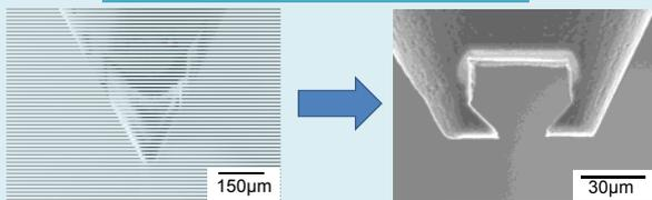
SEM images of the micro-gripper and micro-tensile specimen fabricated by focused ion beam (FIB)
