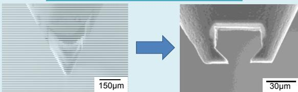
SEM images of the micro-gripper and micro-tensile specimen fabricated by focused ion beam (FIB)
