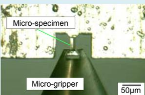
Optical image of the micro-gripper and micro-specimen during the micro-tensile test
